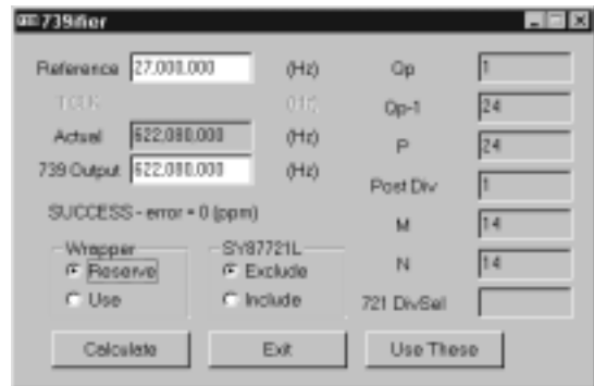
Figure 14. Generating 622.08MHz Without the Wrapper (Using SY87739L only)
